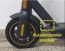
The footrest is attached to the e-scooter, and the rider receives data on their smartphone when using it. The data collected is transmitted to an artificial intelligence server, allowing the user to check whether multiple people are riding or the scooter is driving on the sidewalk in the current state. Once the smartphone app detects tandem riding, the user is sent a push notification on their app.
