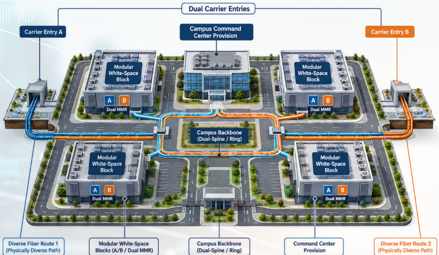
Conceptual camps topology illustrating dual carrier entries, modular white-space blocks, and future command center provisions.
