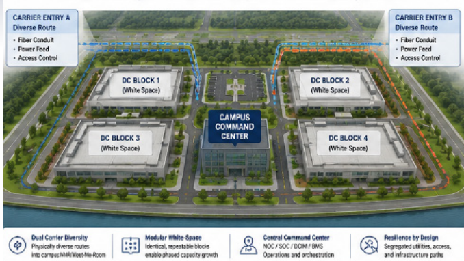
Figure 1. ICT-led data center campus topology with dual carrier entries, modular white-space blocks, and campus command center provisions.
